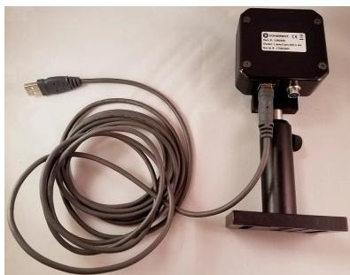
2. If the camera is to be used with an external trigger, connect a 'Y' cable. Connect the camera end by rotating the cable until the orientation matches, and then pushing the connector securely onto the mating connector.
